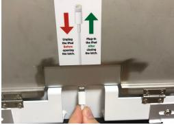
Pass the white cable up through the hole to the Top Piece, and then plug the lightning cable into the iPad as shown on the sticker.
