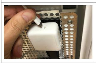
If it is not already, plug the USB-C cable end of the white cable into the power supply in the Middle Piece.
