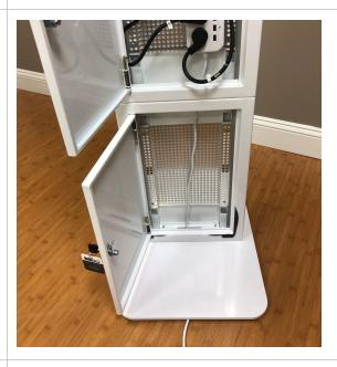
You can then run the AC cable underneath the Baseplate and plug it into an AC outlet. Note: It is easier to do this before attaching the top piece.
