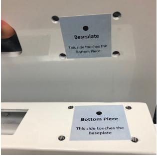
Stand the Bottom Piece up in the foam. To identify the Bottom Piece note that it does not have the two holes in the side and has vents.
