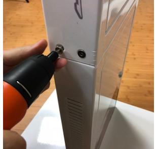
Connect the Middle Piece to the Bottom Piece. The stickers will indicate how they connect. Make sure that the back doors are on the same side.
